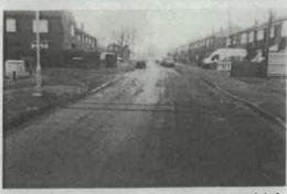
ATC tube survey which consists of a pair of tubes laid across the carriageway which are connected to a data logger that allows reports such as traffic volume, speed and vehicle classification to be generated. This type of count would generally be carried over a 7-day period.
